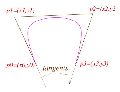
Thus the behaviour of P(t) at the end-points is easily determined from the control polygon:  $P(0) = p_0$  and the tangent  $P'(0) = (p_1 - p_0)/n$ .
