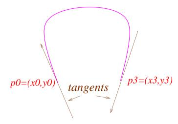
Thus the behaviour of P(t) at the end-points is easily determined from the control polygon:  $P(0) = p_0$  and the tangent  $P'(0) = (p_1 - p_0)/n$ .
