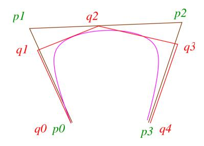
Thus, the control polygon Q may be obtained as an appropriate interpolation of the control-polygon P.
