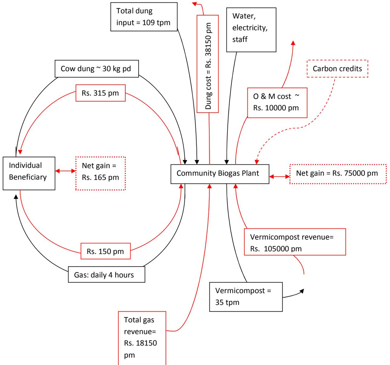
Fig. 2.8 Cash and material flows (Numbers based on operations data)
