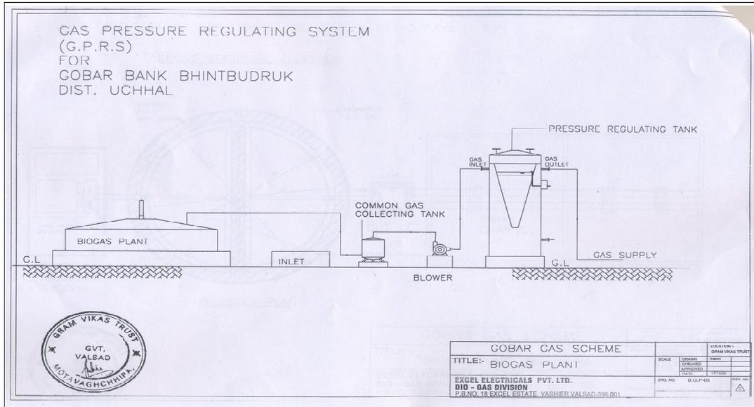
Fig 2.5 Pressure regulation system
