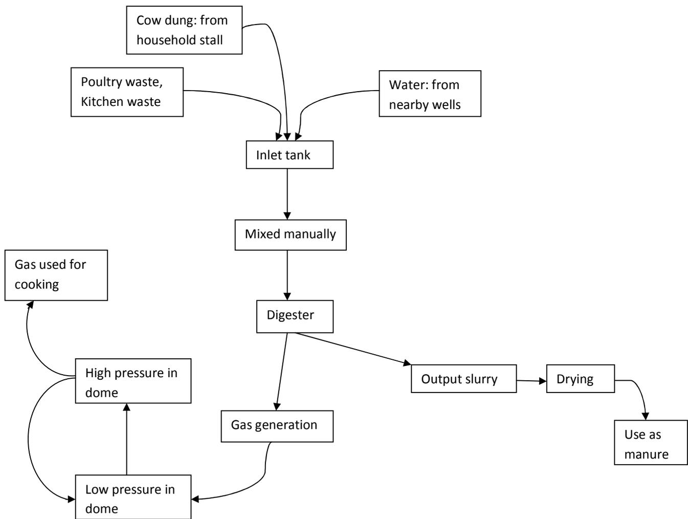
Fig. 3.6 Daily operation of the individual biogas plant
