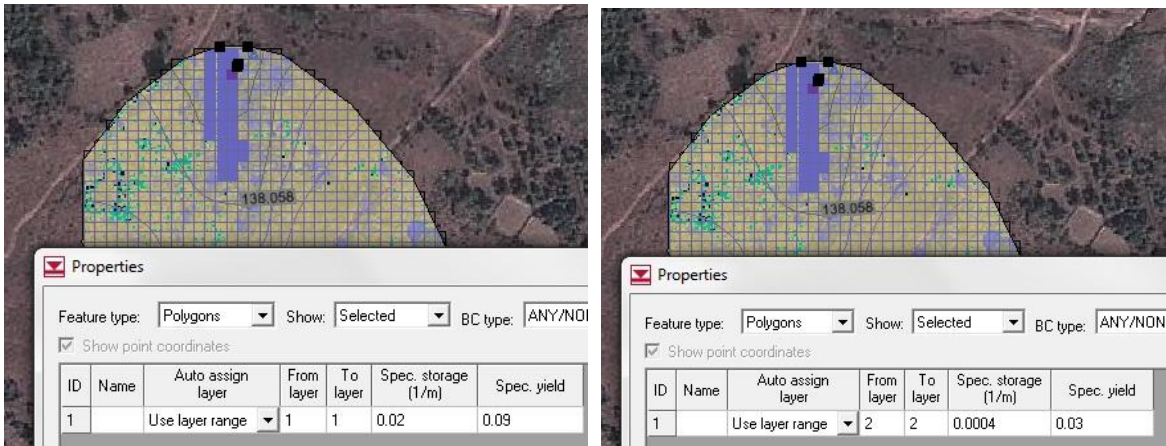
Figure 6-15 – Specific yield and storage values for layer 1 and layer 2
