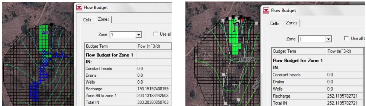
Figure 6-23 – Flow budget at the end of steady state– impact of intervention
