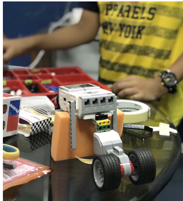
Fig. 5. An intermediate design by group 1 with two wheels and a single motor.
