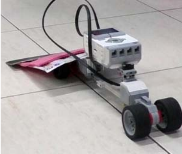
Fig. 2. A four-wheel cleaning robot designed by group 1.
