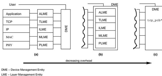
**Figure 4. Cross layer architecture**
