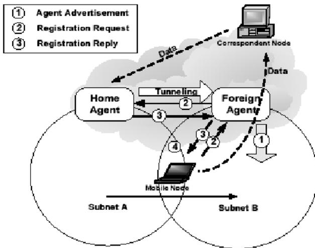
Fig. 1. Working of Mobile IP
