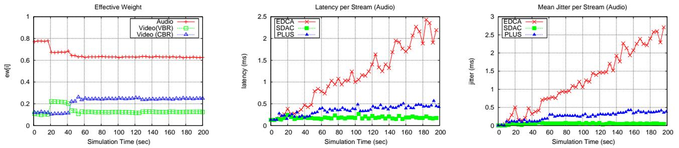
Fig. 3. Variation of  $ew[i]$  and Audio latency characteristics
