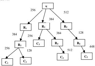
$S: Source \\ R_1, R_2, ... R_n: relay nodes \\ C_1, C_2, ... C_n: clients \\ \\ C_1 = 512 \text{ kbps} \\ T=1 \text{ hour}$
