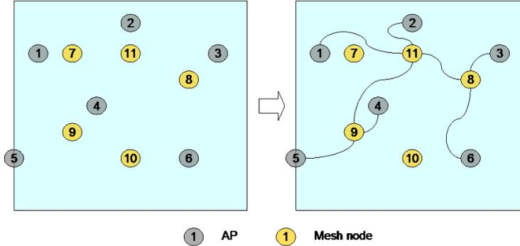
Figure 2: (a) 6 AP, 5 mesh node deployment scenario. (b) Output topology for a power-based cost function.
