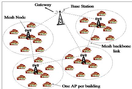
Figure 1: A typical mesh network scenario.
