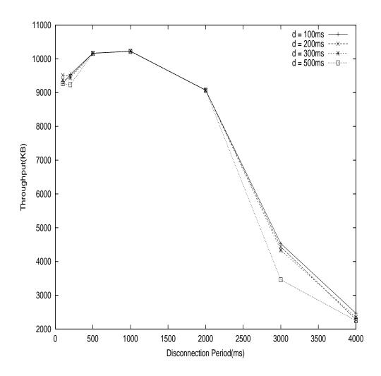
$\diamond$  FH to MH: ATCP throughput for various value of variable d
