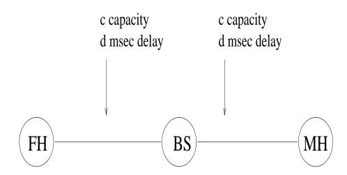
For Simulating WLAN c = 10 Mbpsd = 1 msec
