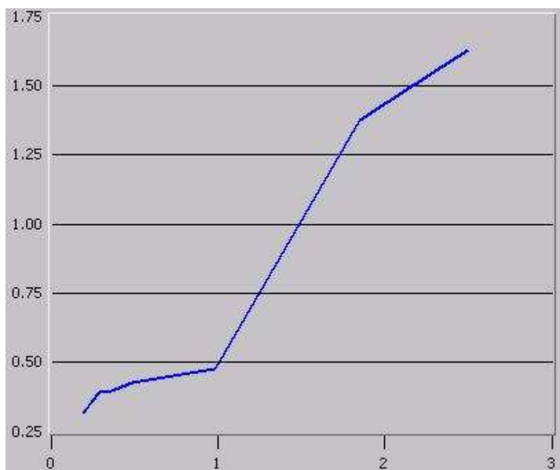
Figure 6.4: Throughput vs Delay of BE flows. Y-axis is in seconds, X-axis in 10Mbps
