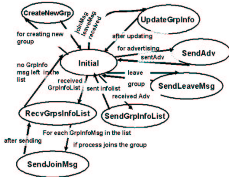
Figure 5.1: Group Join/Leave Protocol state diagram
