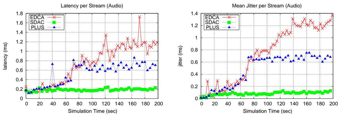
Figure 6.12: Audio latency characteristics
