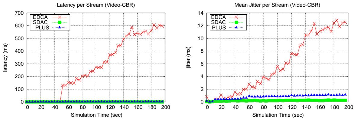
Figure 6.4: CBR latency characteristics
