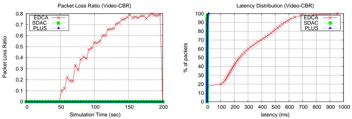
Figure 6.7: CBR packet loss and latency distribution
