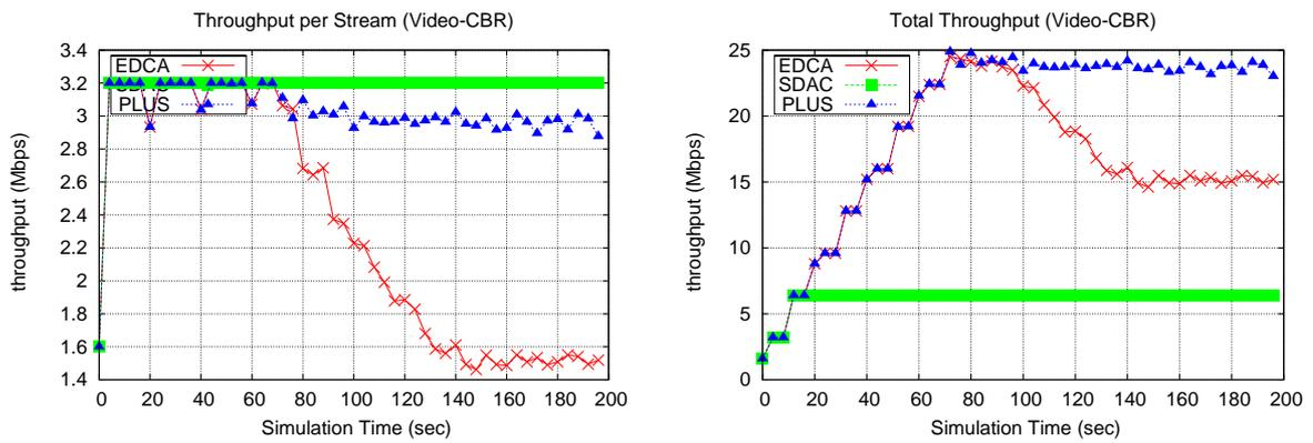
Figure 6.16: Video throughput characteristics
