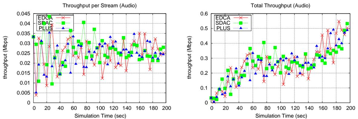
Figure 6.8: Audio throughput characteristics
