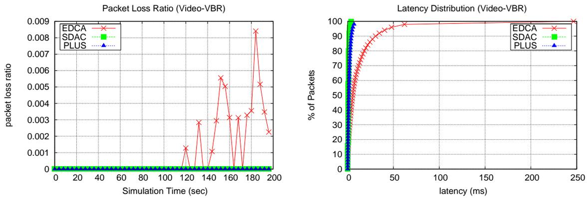
Figure 6.6: VBR packet loss and latency distribution
