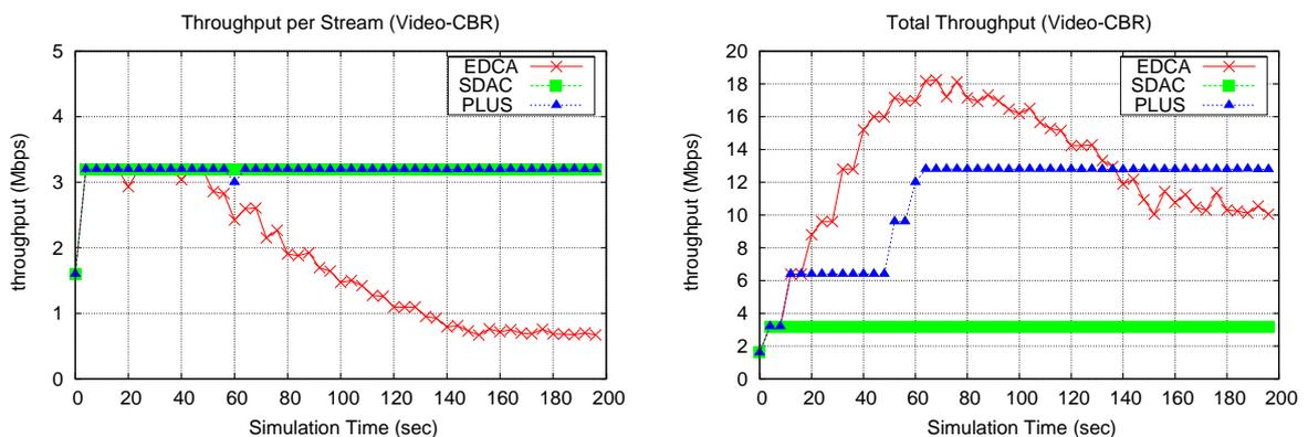
Figure 6.10: CBR throughput characteristics
