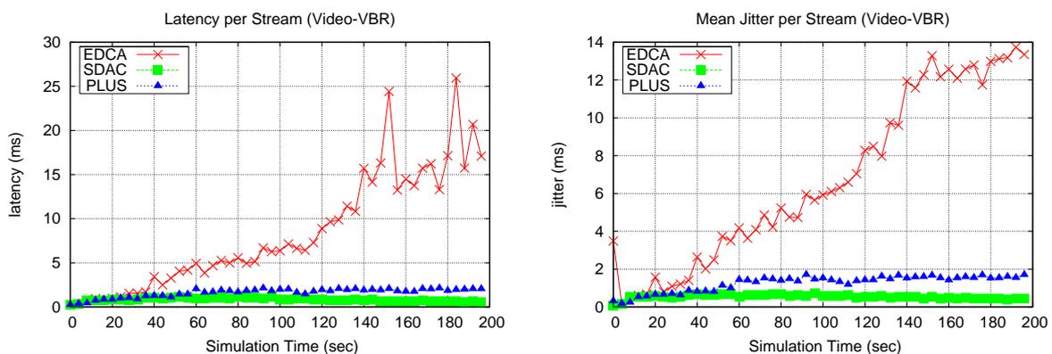
Figure 6.3: VBR latency characteristics
