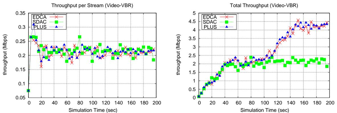
Figure 6.9: VBR throughput characteristics
