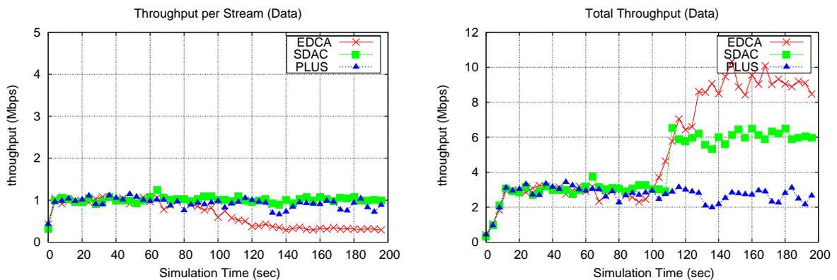
Figure 6.17: Data throughput characteristics
