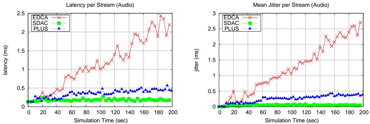
Figure 6.2: Audio latency characteristics
