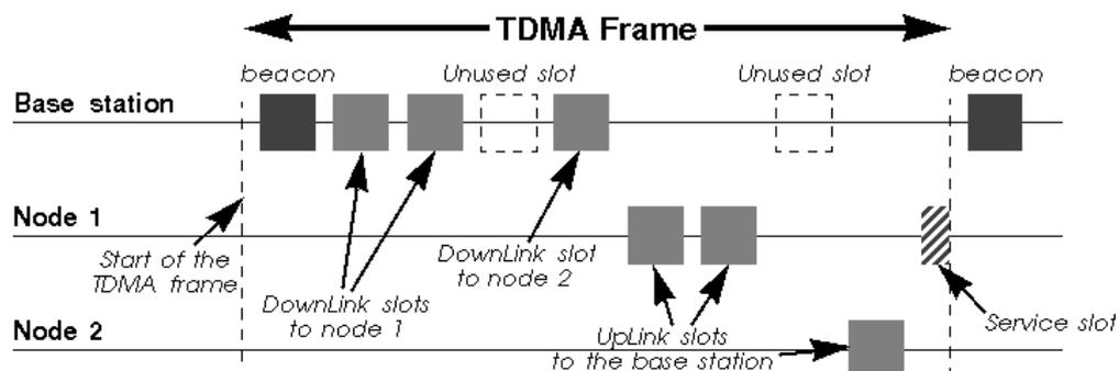
Figure 2.1: TDMA channel Access Mechanism
