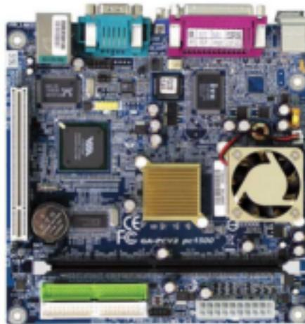
Figure 2.8: Effective motherboard from VIA: VIA PC1500
