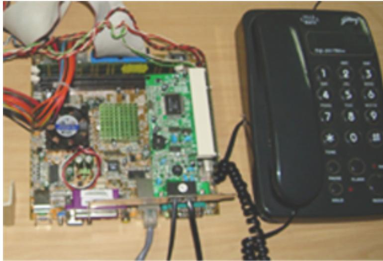
Figure 4.3: Feasible and affordable solution to VoIP Gateway PBX
