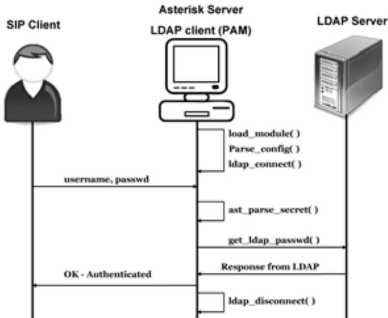
Figure 5.3: Sequence diagram of LDAP authentication in Asterisk
