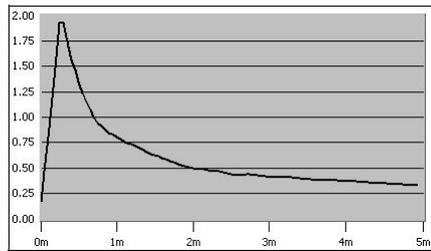
Figure 5.21: End to end delay of rtPS
