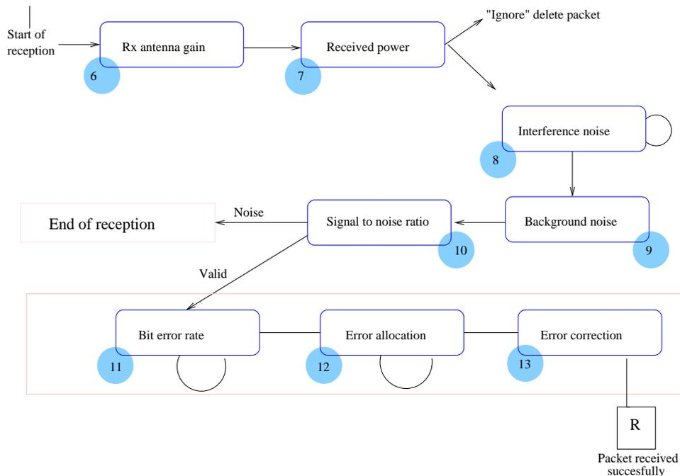
Figure 4.7: Receiver pipeline stages
