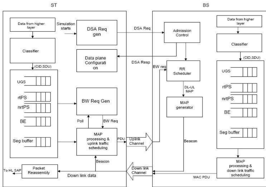
Figure 4.1: WiFiRe Model design block diagram
