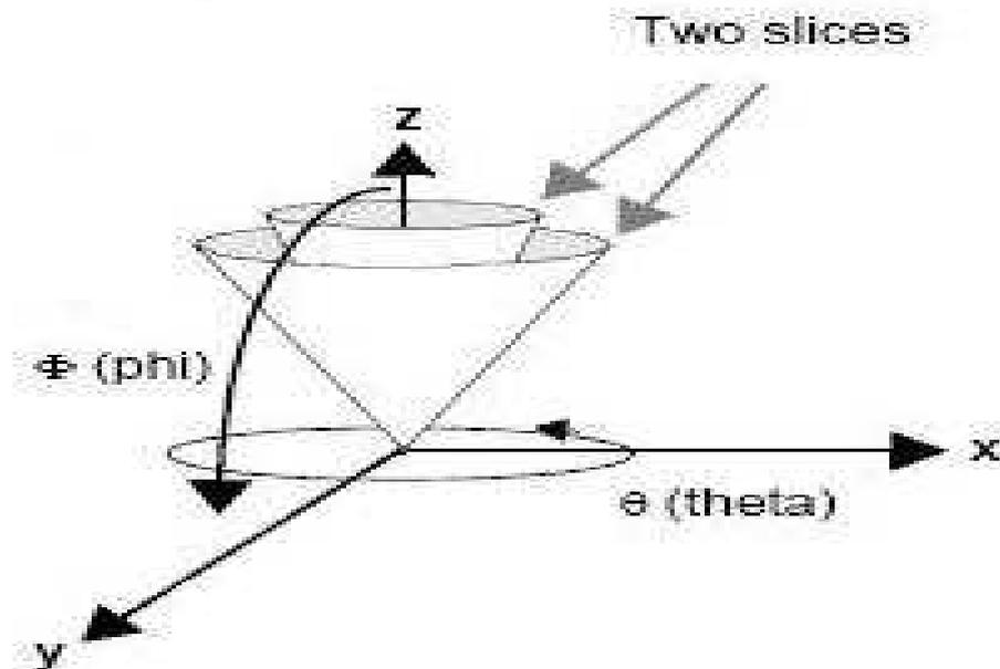
Figure 4.4: Antenna pattern using spherical angles phi and theta
