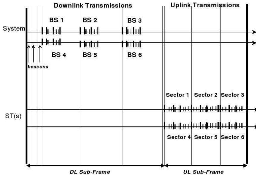
Figure 3.2: Parallel transmission in a six sector system [2]
