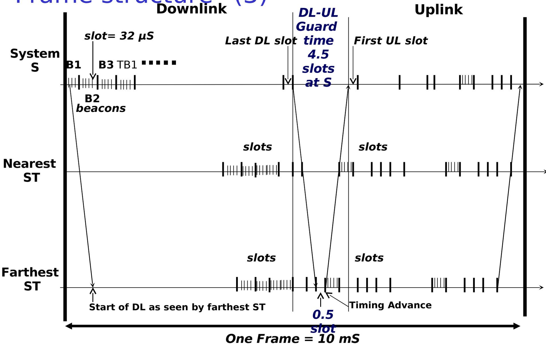
Showing 4.5 slots DL-UL guard time at S. Not to scale.
