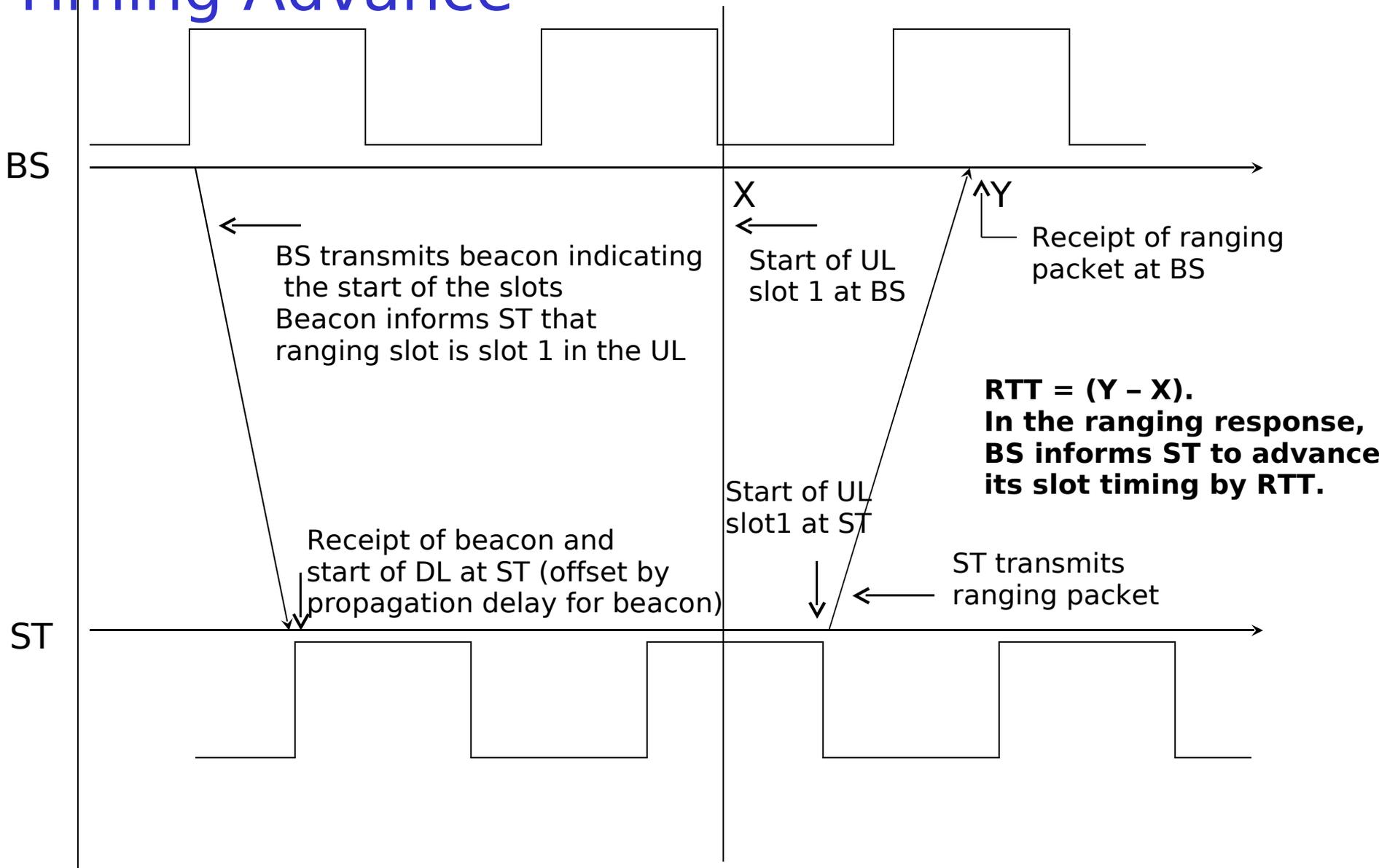
Physical clock pulse durations of BS and ST are synchronized by PHY preamble
