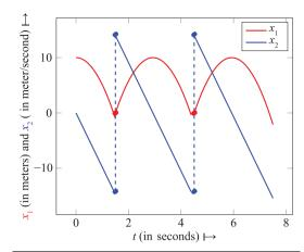
**Figure 7:** A run of the system where the initial vertical position is  $\ell = 10$  meters and the coefficient of restitution c = 1.
