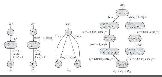
**Figure 8:** Network of hybrid automata  $\mathcal{H}_{j1}$ ,  $\mathcal{H}_{j1}$ , and  $\mathcal{H}_{m1}$  corresponding to jobs  $j_1$  and  $j_2$ , and a machine  $m_1$ , and their product automata  $\mathcal{H}_{i1} \otimes \mathcal{H}_{i2} \otimes \mathcal{H}_{m1}$ .
