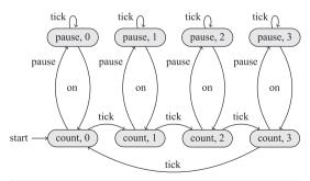
Figure 1: State transition graph for a mod-4 counter.
