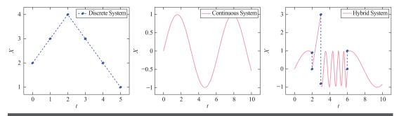
Figure 5: Runs of discrete, continuous, and hybrid systems
