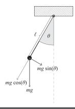
**Figure 3:** An idealized pendulum with length I and mass m.
