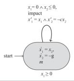
Figure 6: A hybrid automaton modeling the dynamics of a bouncing ball.
