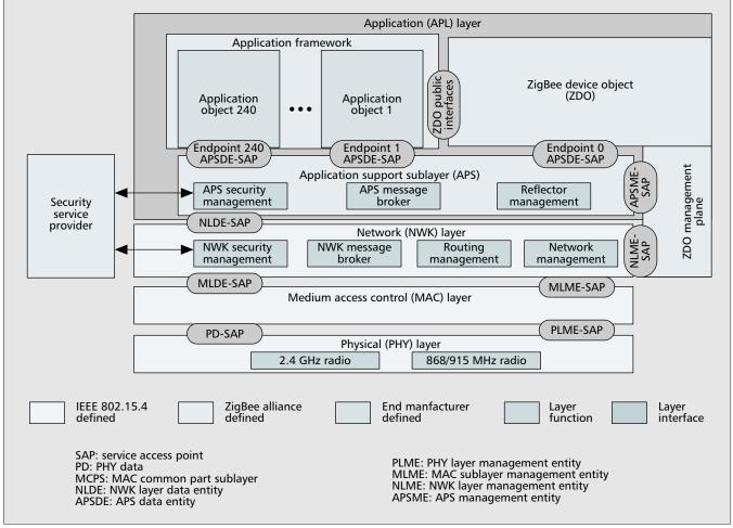
■ Figure 6. ZigBee stack architecture.
